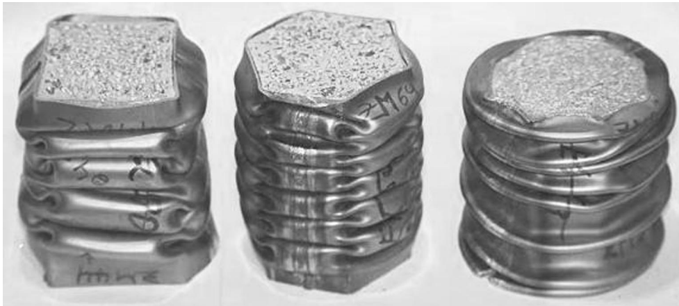
Fig. 6. Series Z: square, hexagonal and octagonal monotubal crushed specimens ZM44 ( \rho_f = 0.47 \text{ g/cm}^3 ), ZM64 ( \rho_f = 0.47 \text{ g/cm}^3 ), ZM83 ( \rho_f = 0.58 \text{ g/cm}^3 ).
