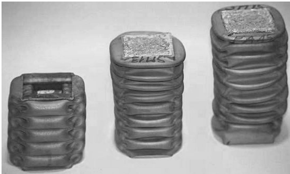
Fig. 4. Series S: empty and monotubal crushed specimens SEM2, SM13 ( \rho_r = 0.43 \text{ g/cm}^3 ), SM15 ( \rho_r = 0.68 \text{ g/cm}^3 ).
